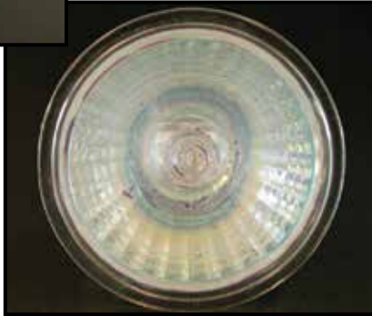
Brand X – Standard dichroic reflector C-6 filament coating has cracked and degraded after only 3000 hours
