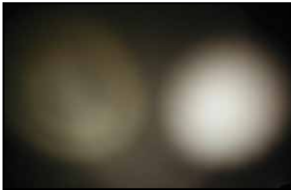
Brand X – Uneven beam pattern, low color temperature, green color and low output
