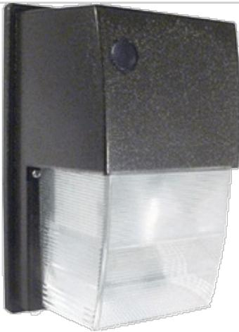
28 thru 42 Watt compact fluorescent Tallpack. Vandal resistant polycarbonate housing. Heavy die-cast aluminum back plate with 1/2" bottom and back conduit opening. Factory installed 120V photocell with bypass cap included. Operating temperature 28w (-20°F), 26, 32 & 42w(0°F). Lamp supplied.
