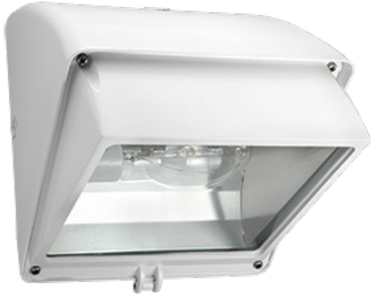
Cutoff Wallpack with glare shield for 35 - 100W HPS, 50 - 100W MH (Pulse Start Standard) or 42W CFL. Lens is flat, tempered glass. 30°. cutoff strip included. Lamp supplied.
