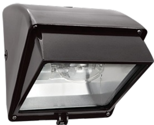
Cutoff Wallpack with glare shield for 35 - 100W HPS, 50 - 100W MH (Pulse Start Standard) or 42W CFL. Lens is flat, tempered glass. 30°. cutoff strip included. Lamp supplied.
