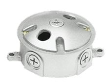
Die cast aluminum wiring box with weatherproof gasket, ground screw, and two sturdy lugs for wall or ceiling mounting. Die cast aluminum cover with three 1/2" holes supplied with 2 stainless steel screws and one close-up plug.
