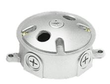
Die cast aluminum wiring box with weatherproof gasket, ground screw, and two sturdy lugs for wall or ceiling mounting. Die cast aluminum cover with three 1/2" holes supplied with 2 stainless steel screws and one close-up plug.
