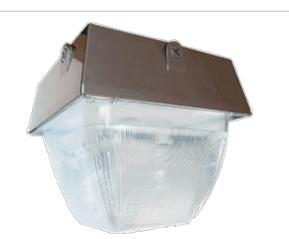
Large size ceiling mount fixture: Horizontal CFL lamps. "No Bend" conduit entrance. Housing is die cast aluminum with clear vandalproof polycarbonate refractor. Available with Emergency Battery Backup option with 42 Watt. Lamp supplied
