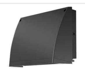
37, 57 and 62 Watt SLIM Wallpacks are designed to cover the footprint of most traditional wallpacks. They are suitable for mounting heights from 20' to 30', and replace HID Wattages from 200W MH to 320W MH. These ultra-high efficiency fixtures are available in cutoff or full cutoff models.
