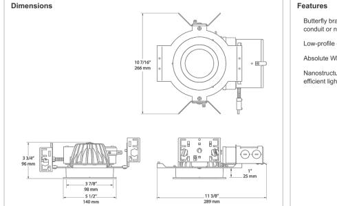
Butterfly bracket allows mounting with bar stock, "C" channel, 1/2" conduit or nailer bars
