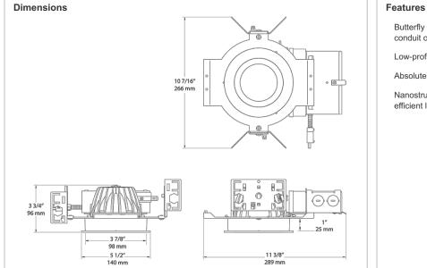
Butterfly bracket allows mounting with bar stock, "C" channel, 1/2" conduit or nailer bars
