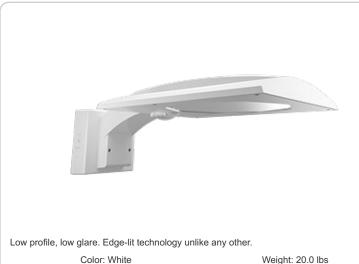
Project: Type: Prepared By: Date: **Driver Info** LED Info 67W Type: Constant Current Watts: 120V: 0.58A Color Temp: 5000K (Cool) 208V: 0.34A Color Accuracy: 75 CRI 240\/-0.29A L70 Lifespan: 100,000 277V: 0.25A 7.608 Lumens: Input Watts: 70W Efficacy: 109 LPW Efficiency: 96%
