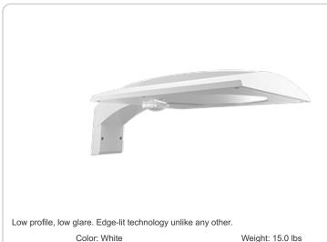
Project: Type: **Prepared By:** Date: **Driver Info** LED Info Constant Current 67W Type: Watts: 120V: N/A Color Temp: 5000K (Cool) 208V: N/A Color Accuracy: 75 CRI 240\/-N/A L70 Lifespan: 100,000 277V: N/A Lumens: 8.146 Input Watts: 69W Efficacy: 119 LPW Efficiency: 98%
