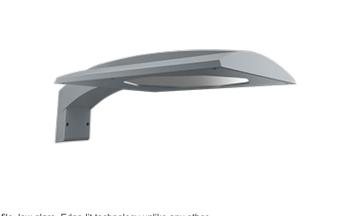
Project: Type: **Prepared By:** Date: **Driver Info** LED Info Constant Current 67W Type: Watts: 120V: 0.58A Color Temp: 5000K (Cool) 208V: 0.34A Color Accuracy: 75 CRI 240\/-0.29A 100,000 L70 Lifespan: 277V: 0.25A Lumens: 7.608 Input Watts: 70W Efficacy: 109 LPW Efficiency: 96%
