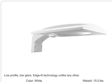
Project: Type: **Prepared By:** Date: **Driver Info** LED Info Constant Current 67W Type: Watts: 120V: 0.58A Color Temp: 3000K (Warm) 208V: 0.34A Color Accuracy: 80 CRI 240\/-0.29A L70 Lifespan: 100,000 277V: 0.25A Lumens: 6.422 Input Watts: 66W Efficacy: 97 LPW Efficiency: N/A
