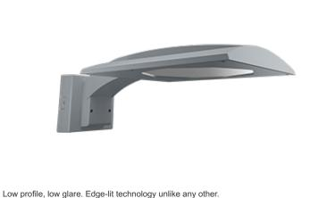
Project: Type: **Prepared By:** Date: **Driver Info** LED Info Constant Current Watts: 67W Type: 120V: N/A Color Temp: 3000K (Warm) 208V: N/A Color Accuracy: 80 CRI 240\/-N/A L70 Lifespan: 100,000 277V: N/A Lumens: 8.158 Input Watts: 73W Efficacy: 112 LPW Efficiency: 92%
