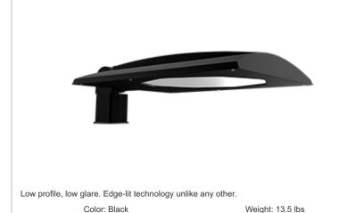
Project: Type: **Prepared By:** Date: **Driver Info** LED Info Constant Current 67W Type: Watts: 120V: N/A Color Temp: 4000K (Neutral) 208V: N/A Color Accuracy: 73 CRI 240\/-N/A L70 Lifespan: 100,000 277V: N/A Lumens: 8.140 Input Watts: 73W Efficacy: 111 LPW
