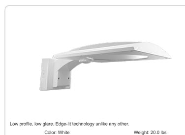
Project: Type: **Prepared By:** Date: **Driver Info** LED Info Constant Current 94W Type: Watts: 120V: 0.83A Color Temp: 3000K (Warm) 208V: 0.48A Color Accuracy: 80 CRI 240\/-0.42A L70 Lifespan: 100,000 277V: 0.36A Lumens: 10.167 Input Watts: 93W Efficacy: 110 LPW Efficiency: N/A
