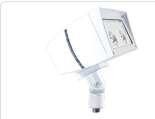
Rectangular shaped LED floodlight designed to replace 250W Metal Halide. Patent Pending airflow technology ensures long LED and driver lifespan. Use for building facade lighting, sign lighting, LED landscape lighting and instant-on security lighting. Weight: 12.6 lbs
