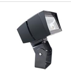
Rectangular shaped LED floodlight designed to replace 175W Metal Halide. Patent Pending airflow technology ensures long LED and driver lifespan. Use for building facade lighting, sign lighting, LED landscape lighting and instant-on security lighting. Weight: 14.2 lbs
