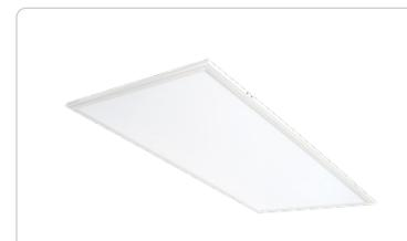
2' x 4' EZPAN edgelit LED panel lights with emergency battery Backup that will operate the LED Lamp for 90 minutes if power fails. For use in drop ceilings or drywall using the optional recessed mounting kit.
