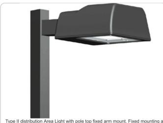
Type II distribution Area Light with pole top fixed arm mount. Fixed mounting at 90° to pole. Drilling 2" on center. Factory wired for 277V. Lamp supplied.
