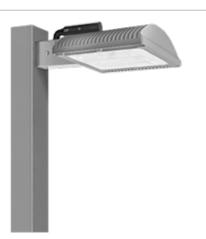
Specification grade area lights available in IES Type III distributions. For use for roadway, general parking and other area lighting applications where a larger pool of lighting is required. Mounts to 4" square steel poles at 20-35'. Patent pending thermal management system. Includes built in support for Lightcloud, a wireless lighting control system and service, fully developed by RAB. 5 Year Warranty.
