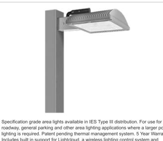
Project: Type: Prepared By: Date: **Driver Info** LED Info Type: Constant Current Watts: 150W 120V: 1.31A Color Temp: 4000K 208V: 0.80A Color Accuracy: 82 CRI 240V: 0.69A L70 Lifespan: 100000 277V: 0.60A 10,106 Lumens: Input Watts: 149W Efficacy: 68 LPW Efficiency: N/A
