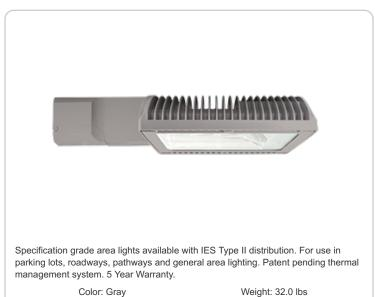
Project: Type: Prepared By: Date: **Driver Info** LED Info Type: Constant Current Watts: 105W 120V: 0.89A Color Temp: 4000K 208V: 0.58A Color Accuracy: 82 CRI 240V: 0.50A L70 Lifespan: 100000 277V: 0.44A 8,377 Lumens: Input Watts: 106W Efficacy: 79 LPW Efficiency: 99%
