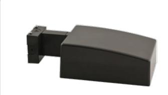
Type II distribution wall mount Area Light with 4" arm for use at 10' - 15' height. Fixed mounting at 90° to wall. Lamp supplied.
